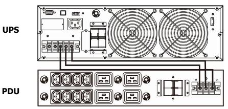
**NOTE:** Make sure that the wires are connected tightly with the terminals. Put the terminal block cover back to the rear panel.
