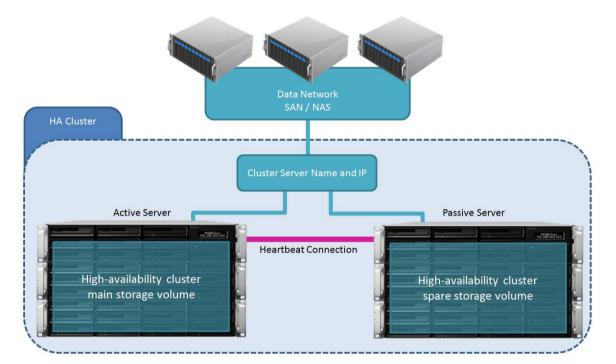
Figure 2: Hosts and NAS clients access a Synology High Availability (SHA) cluster through a single virtual interface
