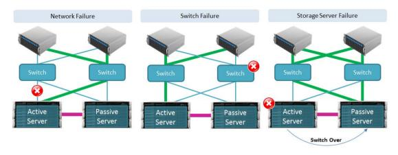
Figure 4: High-availability cluster network configuration on models with four or more LAN ports (iSCSI)
