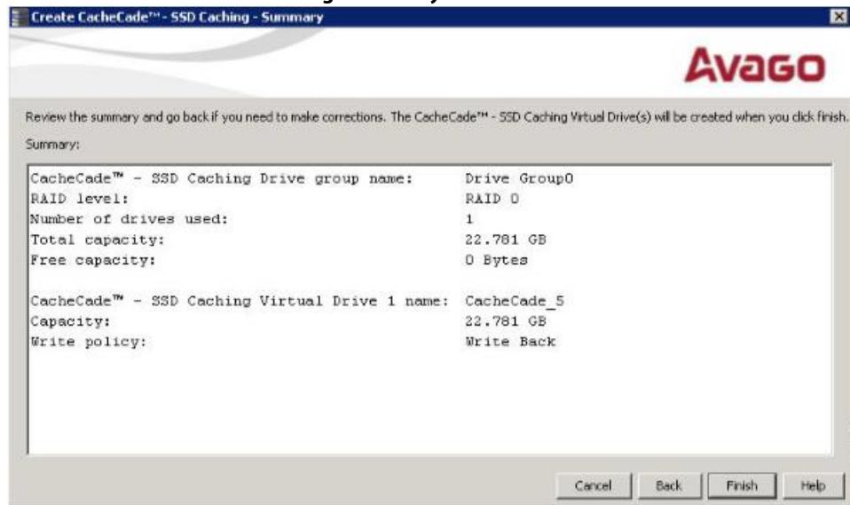
This screen displays the drive group name, the RAID level, the number of drives, the total capacity, the free capacity, the CacheCade virtual drive name, the capacity being used, and the write policy.
