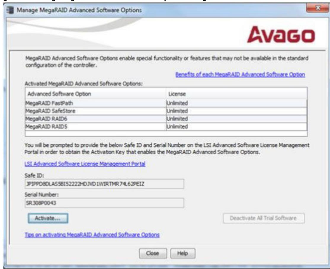
The **Activated MegaRAID Advanced Software Options** table consists of the **Advanced Software Option** and the **License** columns.
