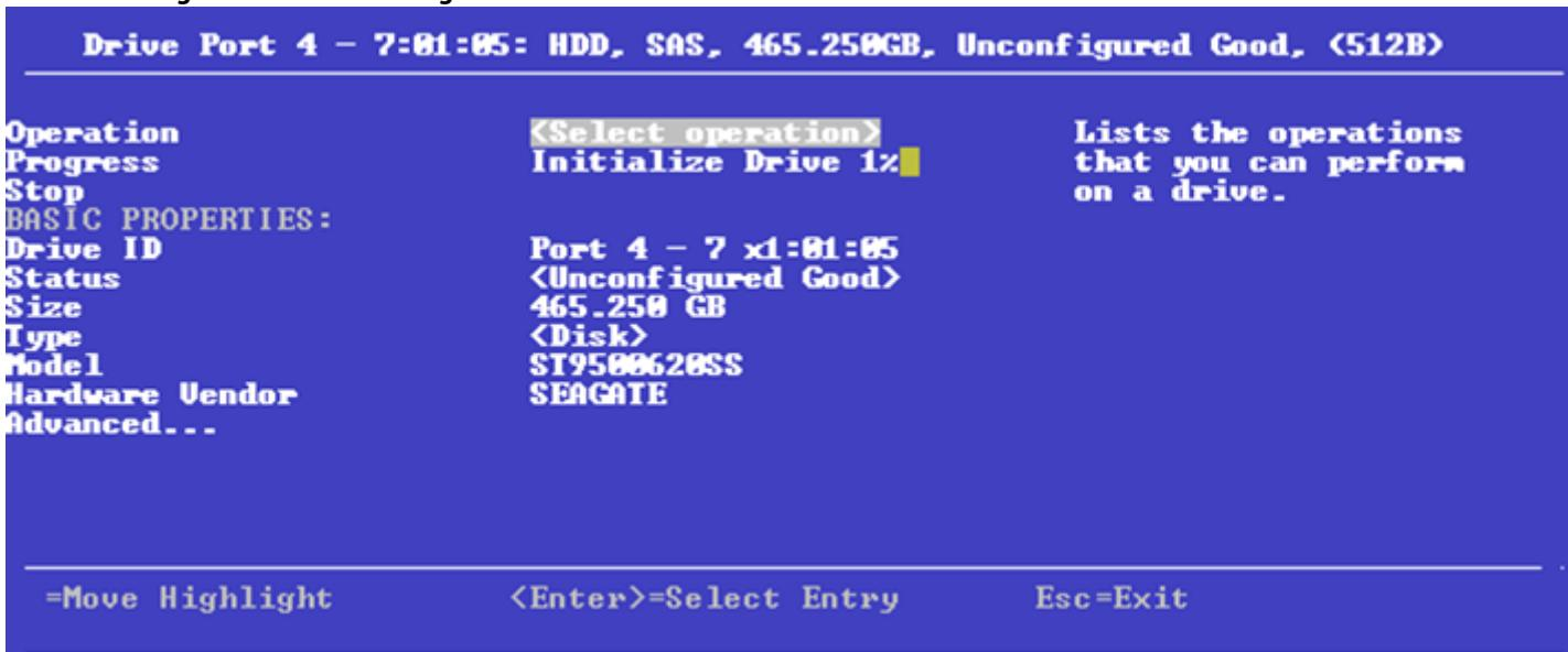
8. To stop the initialization or erase process, highlight **Stop** and press Enter.
