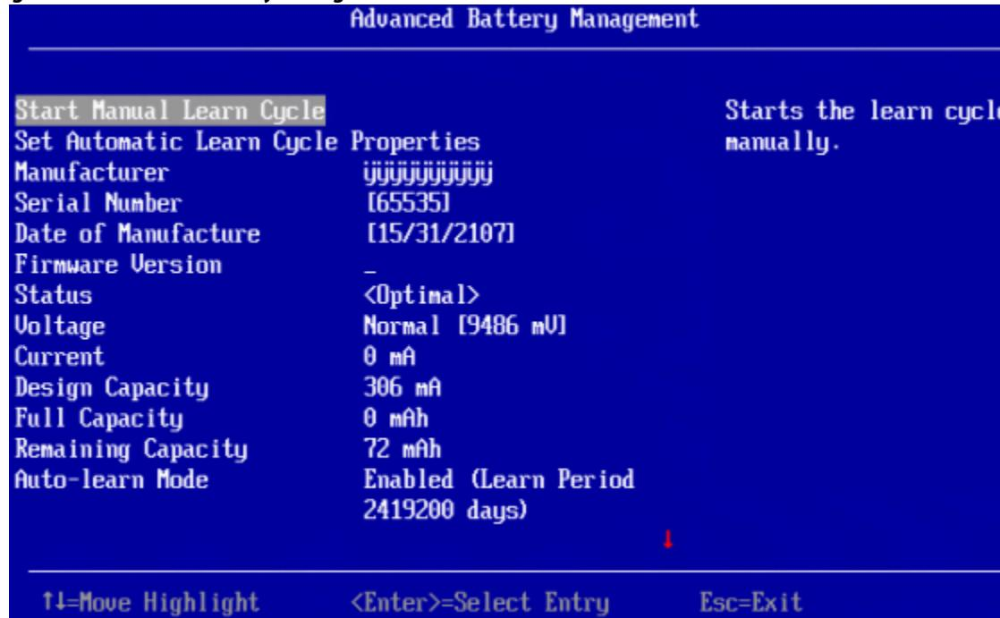
The small red arrow at the bottom of the dialog indicates that you can scroll down to view more Advanced Battery Management properties.
