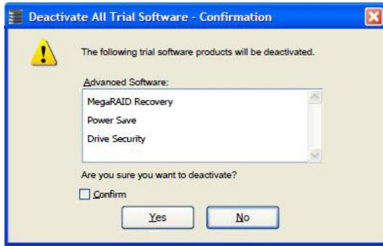
2. Select the **Confirm** check box, if you want to deactivate the software applications, that are used with a trial key.
