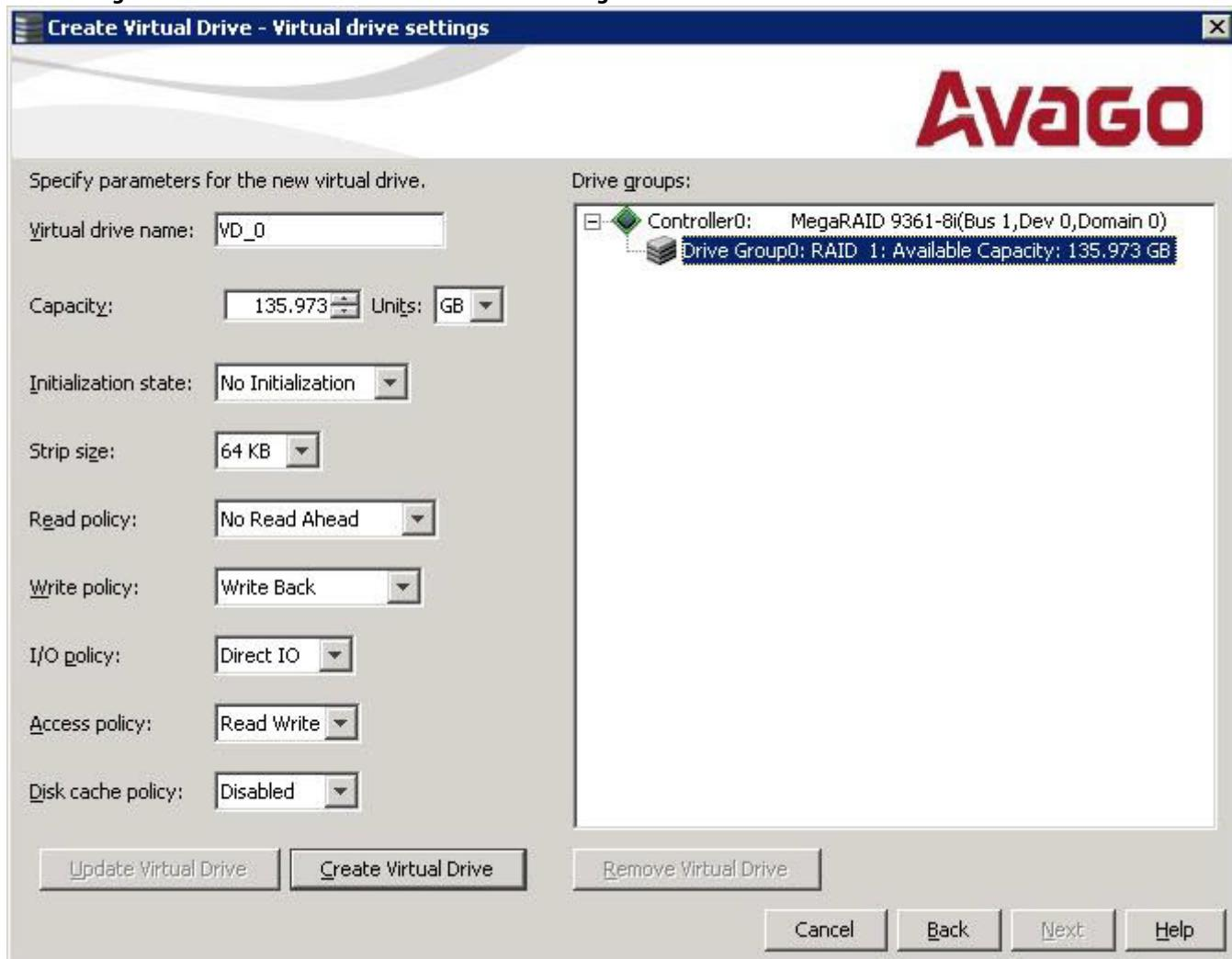
**NOTE** If you select **Write Back** as the write policy, and no battery exists, the battery is low or failed, or the battery is running through a re-learn cycle, the write policy switches to **Write Through**. This setting eliminates the risk of data loss in case of a power failure. A message window notifies you of this change.
