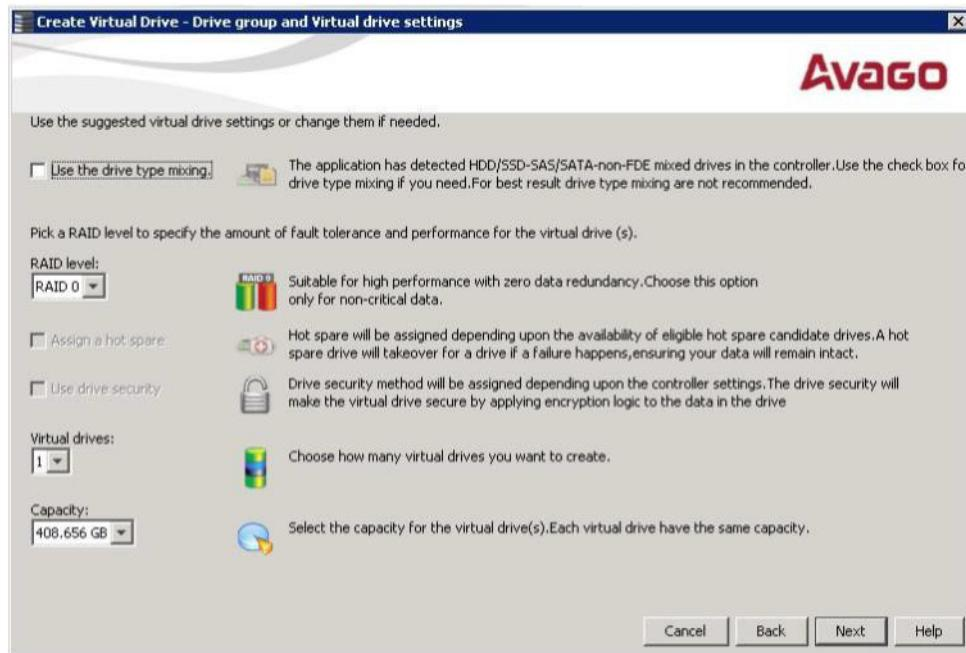
4. If you want to allow different types of drives in a configuration, select the **Use the drive type mixing** check box.
