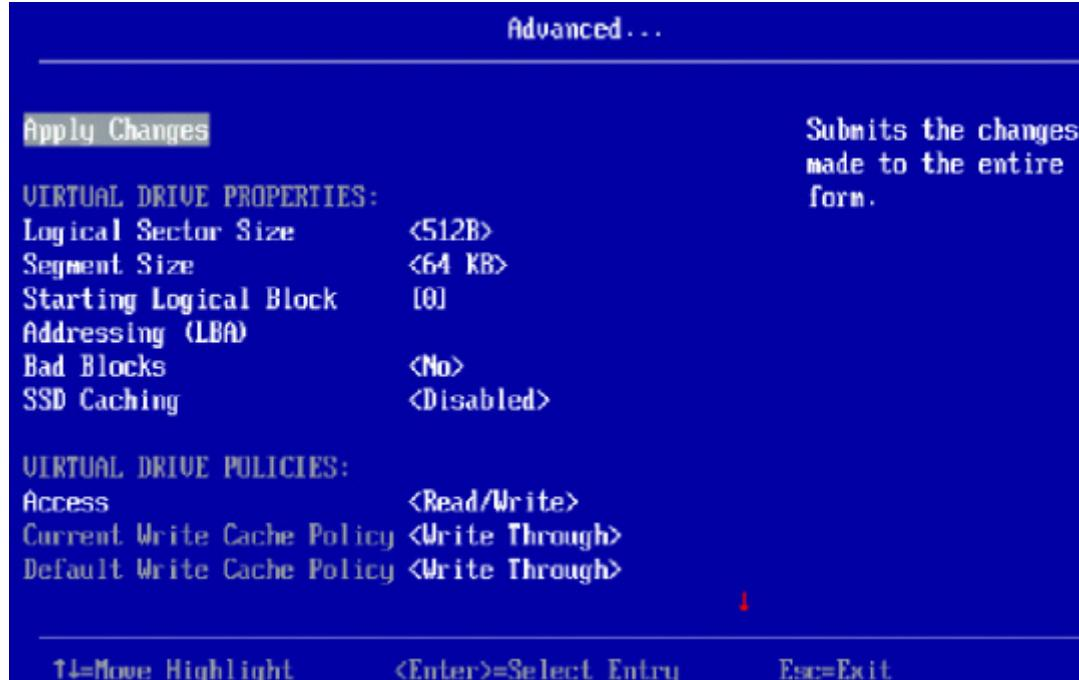
The small red arrow at the bottom of the dialog indicates that you can scroll down to view more virtual drive properties and virtual drive policies, as shown in the preceding figure.
