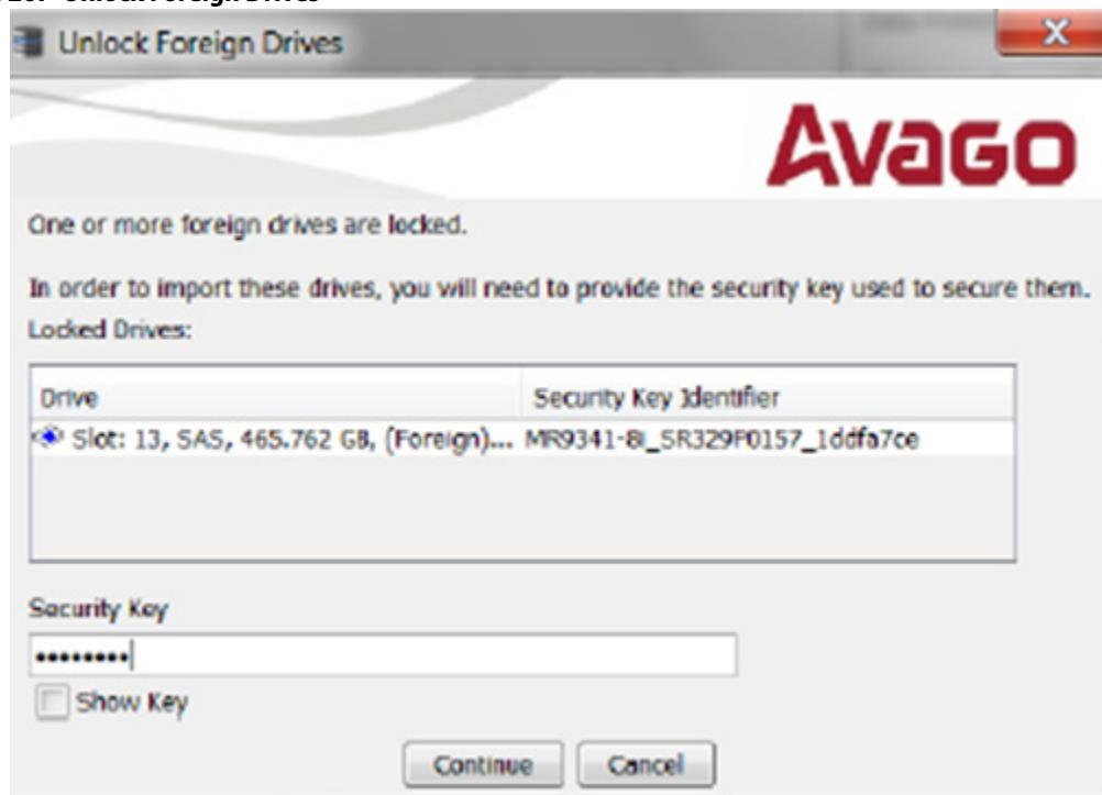
3. Enter the security key to unlock the configuration.
