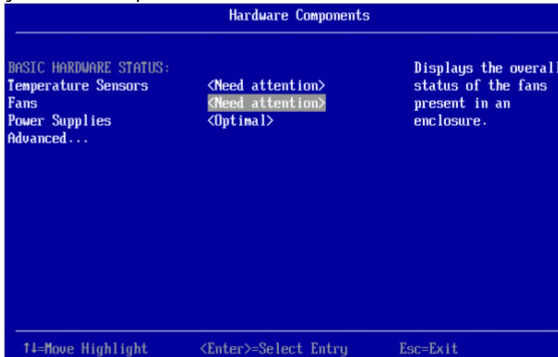
The preceding figure lists the status of the temperature sensors, fans, power supplies, and other hardware components (such as batteries) installed in the system.
