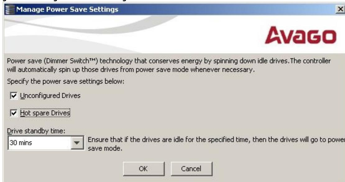
3. Select the **Unconfigured Drives** check box to let the controller enable the unconfigured drives to enter the Power-Save mode.
