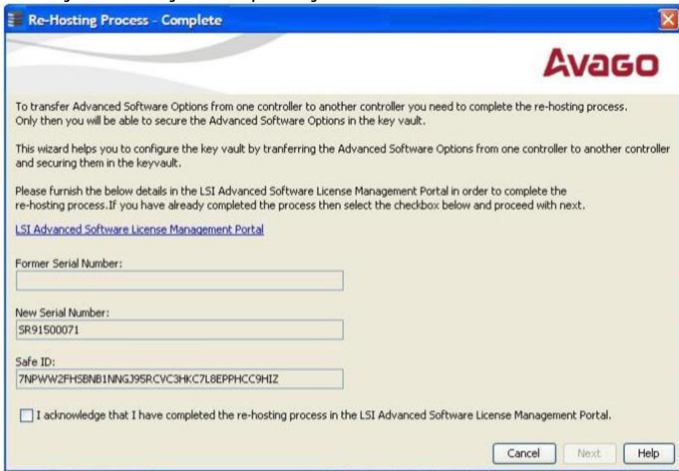
2. Select the **I acknowledge that I have completed the re-hosting process in the LSI Advanced Software License Management Portal** check box if you want to complete the re-hosting process.
