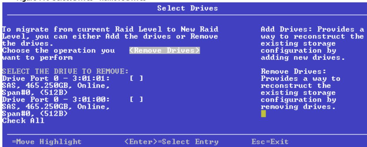
2. To select the drives to remove from the configuration, highlight the drives and press the spacebar. A small red arrow at the bottom of the dialog indicates you can scroll down to view more drives.
