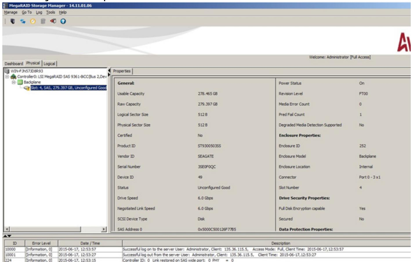
The **Power Status** property displays the status On when a drive is spun up and displays the status Powersave when a drive is spun down. Note that SSD drives and other drives that never spin down still show On.
