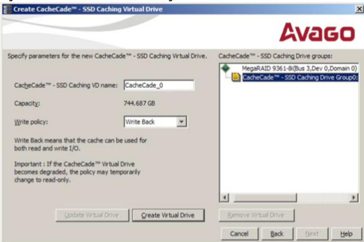
7. Enter a name for the CacheCode virtual drive in the **CacheCode - SSD Caching VD name** field.
