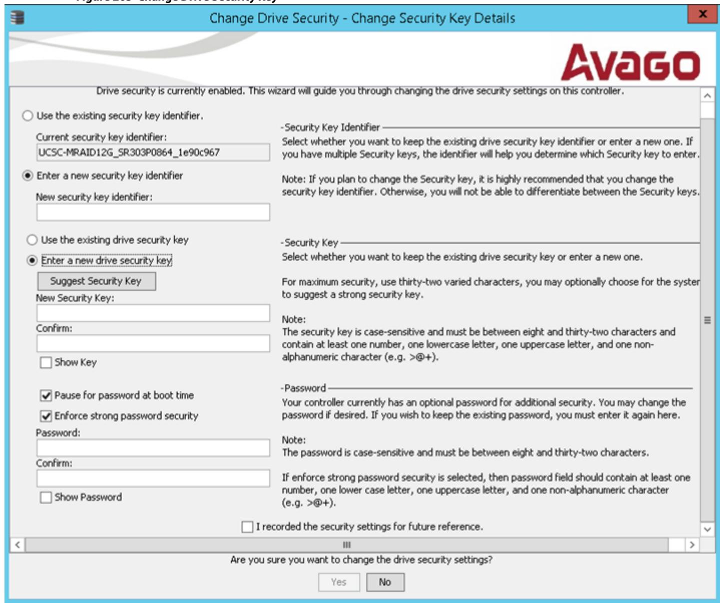
3. Either you can use the existing security key identifier assigned by the controller or specify a new security key identifier.
