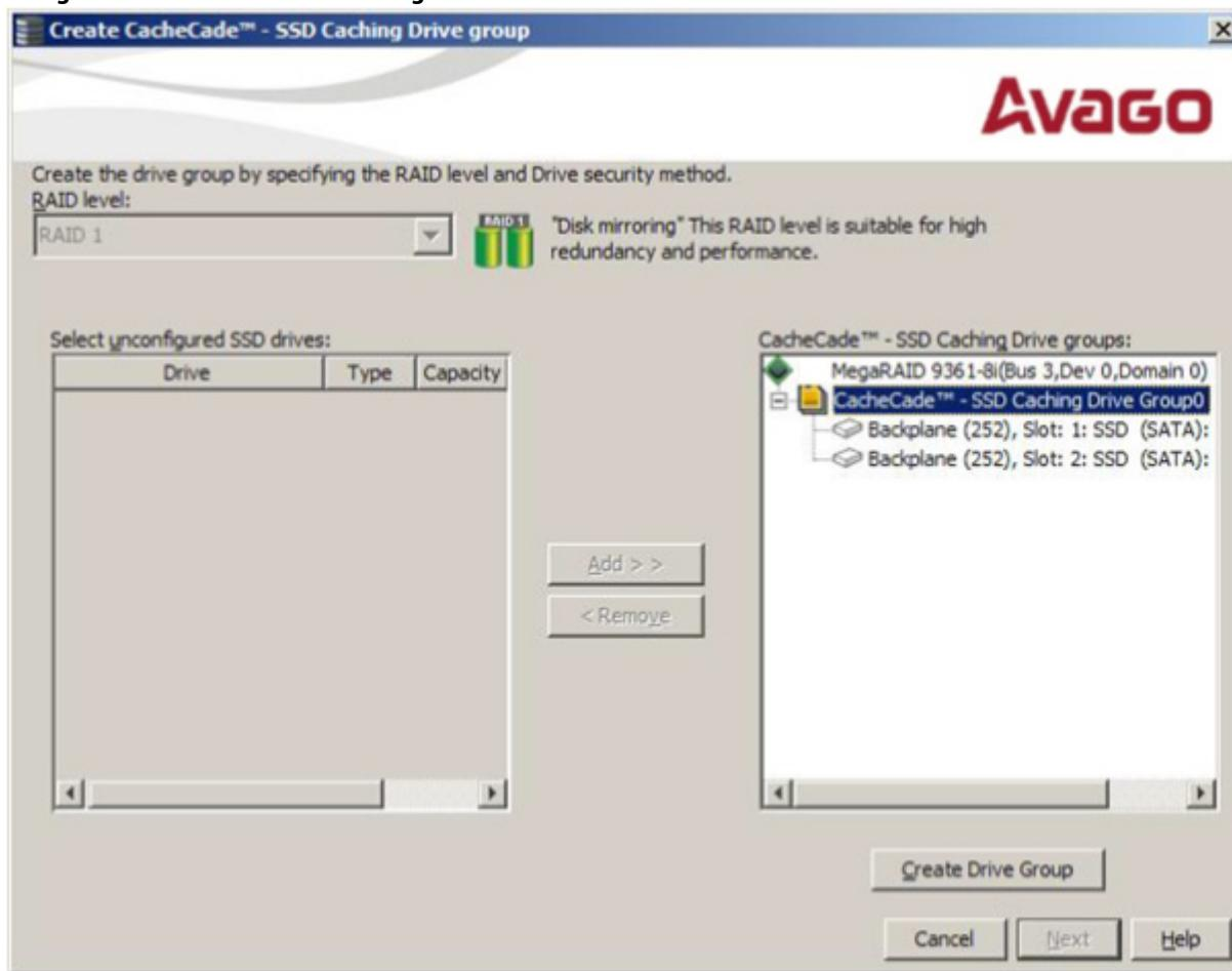
2. Select a RAID level for the CacheCade virtual drive in the **RAID level** field.
