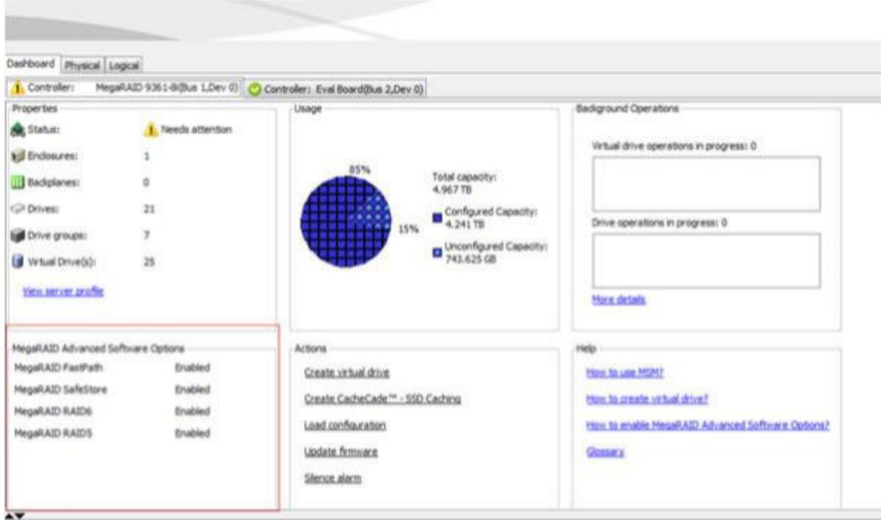
Figure 234 Manage MegaRAID Advanced Software Options Dialog
