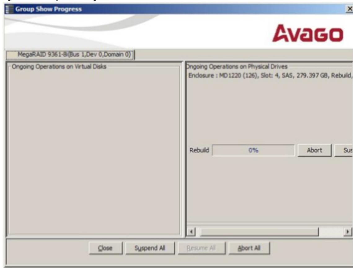
The **Group Show Progress** window displays a percent-complete indicator for drive rebuilds. Rebuilds might take a long time to complete. An up-arrow appears above the drive icon while it is being rebuilt.
