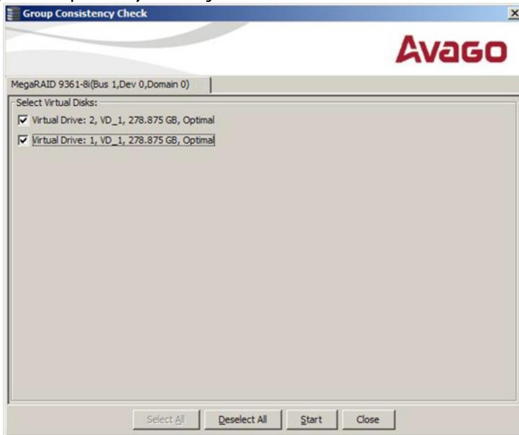
2. Either check the virtual drives on which to run the consistency check, or click **Select All** to select all of the virtual drives.
