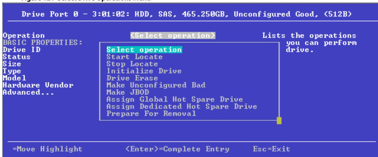
**Start Locate** and **Stop Locate** are the available options for any selected drive. The other menu options vary based on the status of the drive or on the selected personality mode, which can be **Online**, **Offline**, **JBOD**, **Unconfigured Good**, **Unconfigured Bad**, **Global Hot Spare**, and **Dedicated Hot Spare**. If your system is in JBOD personality mode, the **Make JBOD**, **Delete JBOD**, and other personality mode related options appear.
