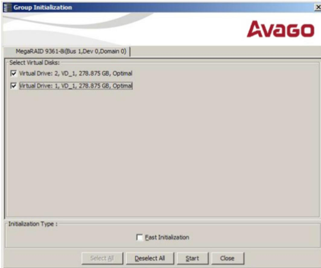
2. Either check the virtual drives on which to run the initialization, or click **Select All** to select all of the virtual drives.
