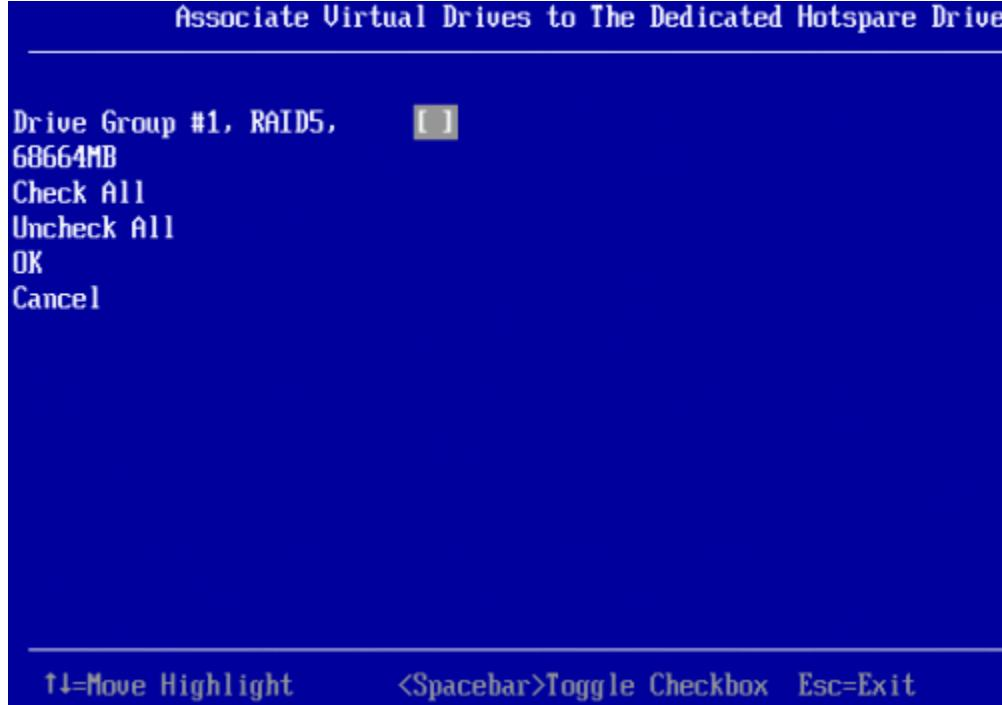
The preceding figure lists a single entry for each existing drive group. If you create a partial virtual drive on the same drive group, you can view a single entry with the cumulative size.
