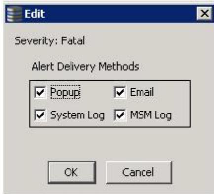
4. Select the desired alert delivery methods for alert notifications at the event severity level.
