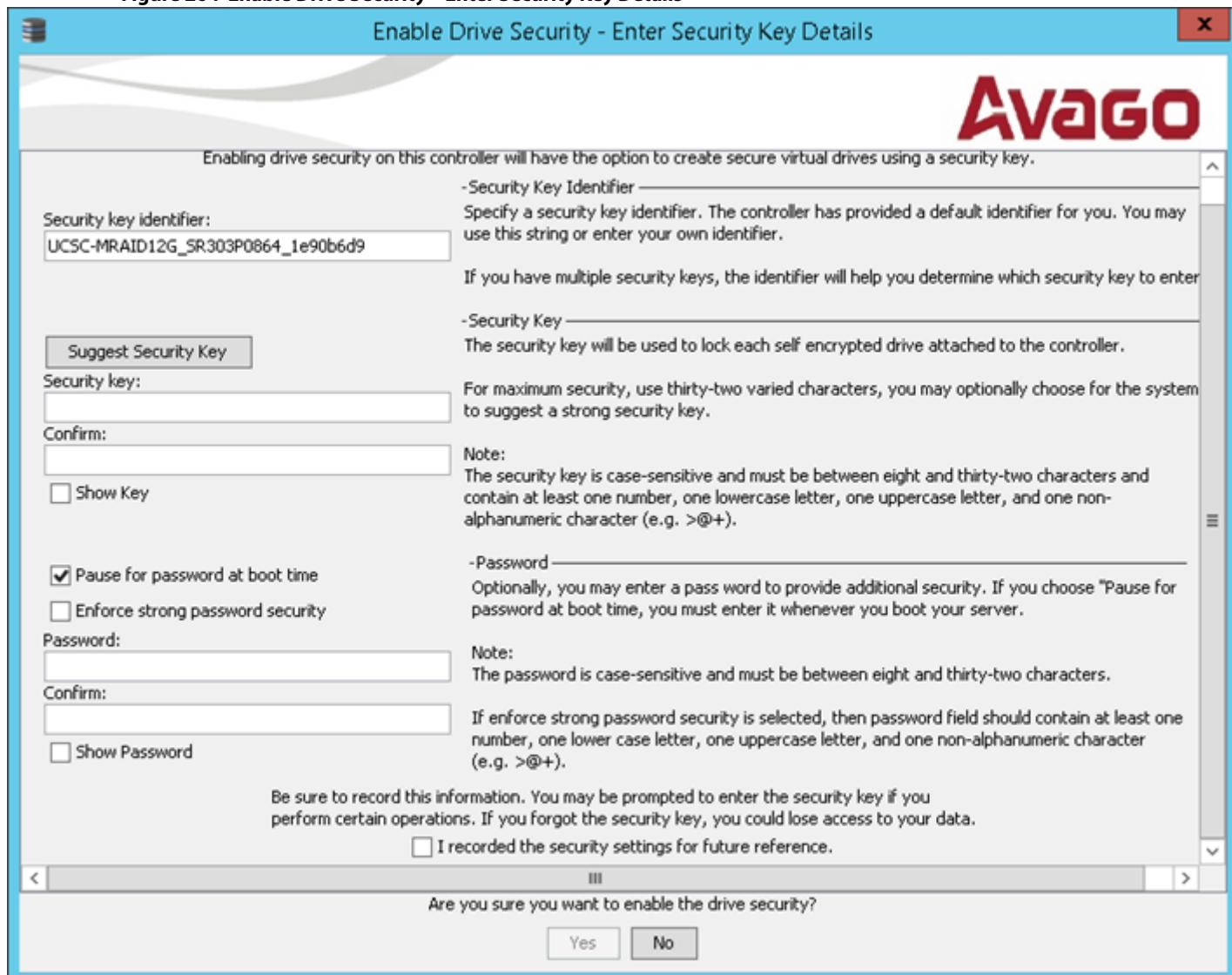
3. Either use the default security key identifier provided by the controller or specify a new security key identifier.
