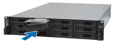
Note: Make sure the tray is pushed in all the way. Otherwise, the drive might not be able to function properly.
