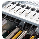
Tool-less adjustable card retainers for full height or low profile cards
