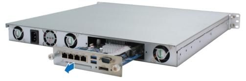
*Important:* When you pull out the panel, you expose sensitive internal components. Avoid touching anything other than the memory assembly when you remove or add memory.
