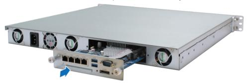
c Tighten the two knobs you unscrewed in step 2.
