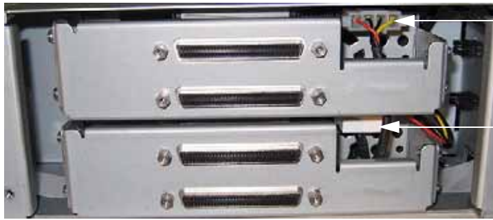
Figure 6 power cable routing— HP half-height SCSI tape drive
