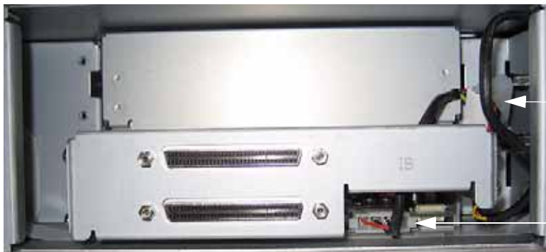
Figure 8 power cable routing—IBM full-height Fibre Channel or SCSI (pictured) tape drive
