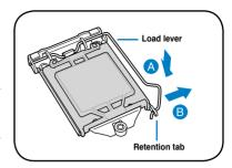
3. Lift the load lever until the load plate is completely lifted.
