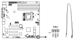
P9D-M Thermal sensor cable connector
