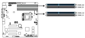
P9D-M 240-pin DDR3 DIMM sockets
