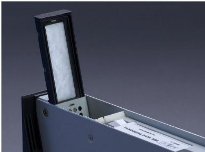
Figure C.1. Replacing dust filter.
