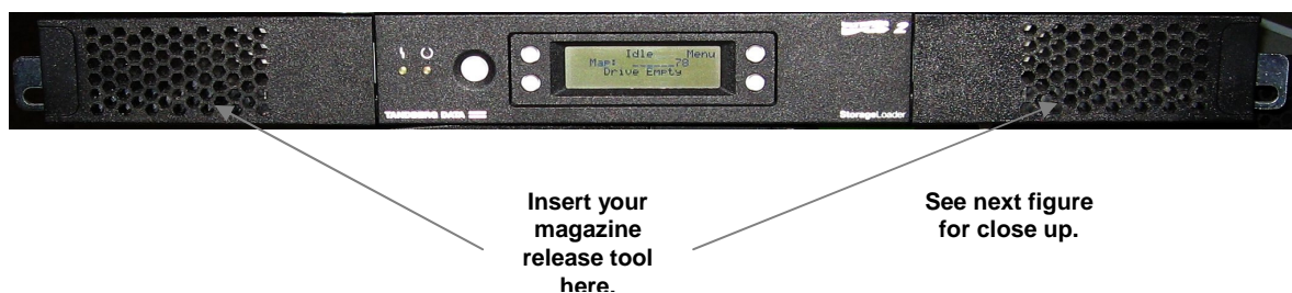
Figure 4.21. Holes used to insert release tool.
