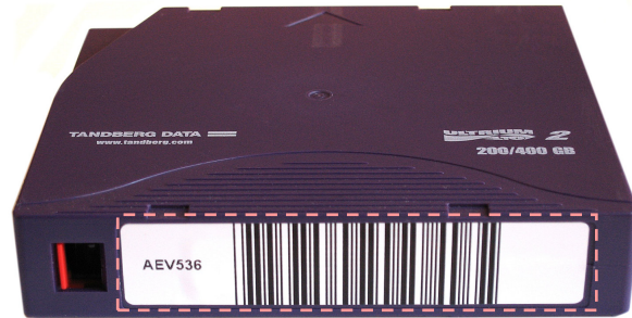
Figure 3.10. Positioning of bar code label for LTO cartridges.
