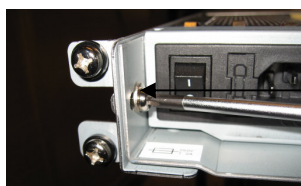
Figure 3.7. Fasten the rear of the StorageLoader to the rails.
