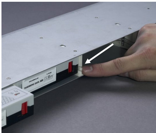
Figure 4.18. Push the release knob towards cartridge to eject.
