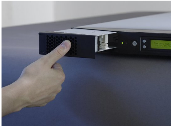
Figure 4.20. Push magazine until it clicks into place.
