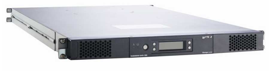
Figure 2.1. Overview of Tandberg Data StorageLoader 1U.
