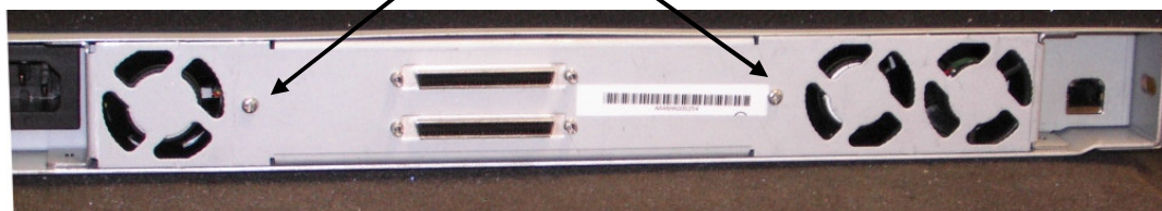
Figure C.8. Replacing the tape-drive.
