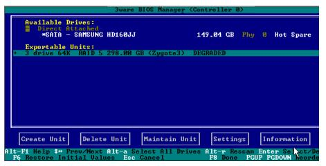
You can start the rebuild of a degraded unit manually in 3BM, or you can let the system boot and allow the rebuild to take place automatically.
