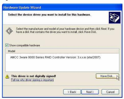
15 When the **Install from Disk** dialog box appears (Figure 86), enter the correct path name to the driver. If you created a driver diskette, insert it now. (The path will be A: if you are using a diskette in the A drive.)
