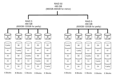
Figure 7. RAID 50 Configuration Example
