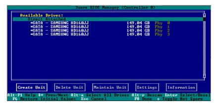
2 After all drives for the unit are selected, **Tab** to the **Create Unit** button and press **Enter**.
