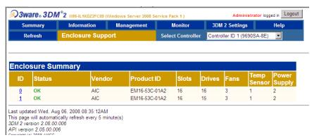
To see details about a particular enclosure, click the link in the ID column. (See "Checking Enclosure Component Status" on page 208)
