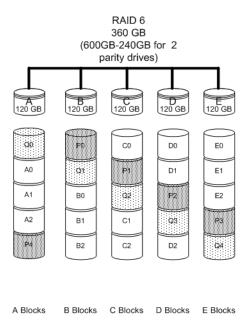
Figure 5. RAID 6 Configuration Example
