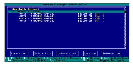
2 After all drives for the unit are selected, use the **Tab** to move to the **Create Unit** button and press **Enter**.
