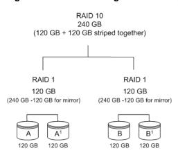
Figure 6. RAID 10 Configuration Example
