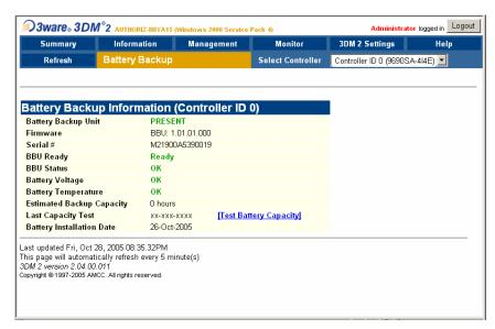
The Battery Backup page appears when you choose **Monitor > Battery Backup** on the menu bar. Use this page to determine whether a backup battery is present, see details about it, and perform a battery test.
