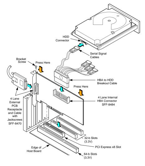
Figure 2.1 Installing an LSI PCIe to SAS x8 HBA in a PCI Express Slot
