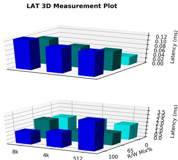
The Latency Measurement 3D Plot shows the average latency on top and the max latency below it. For the measurement window every workload including all block sizes is plotted.
