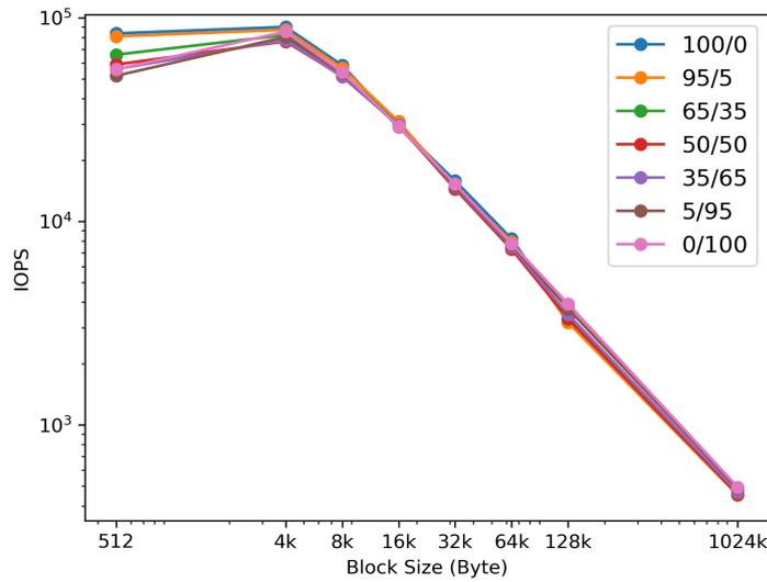
The Measurement Plot shows the average of IOPS in the measurement window. For every workload the IOPS of all block sizes are plotted.
